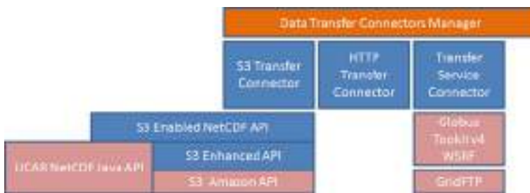
Fig. 26.6 The NetCDF service transfer connector architecture
