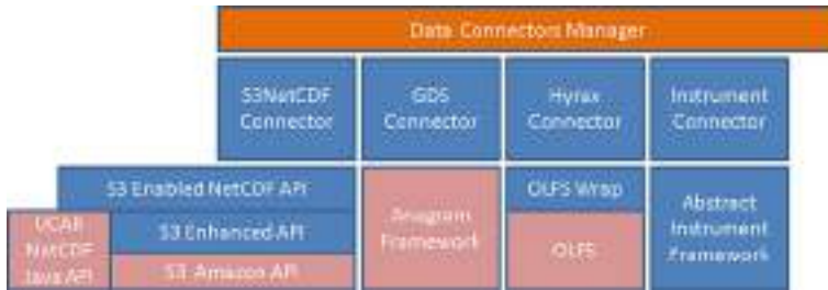
Fig. 26.4 The NetCDF service data connector architecture
