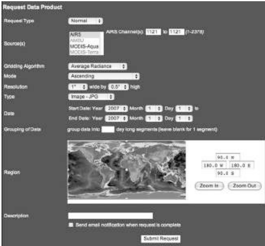
Fig. 16.9 Screenshot of the SOAR system GUI for the gridded average brightness temperature web service.
