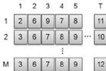
Fig. 12.6 An example chromosome representing a scheduling assignment of (implementation,service type instance) \rightarrow service provider. Each row represents an implementation, and each column represents a service type instance. Here there are M workflows and T service types instances. In workflow 1, any request for service type 3 goes to server 9
